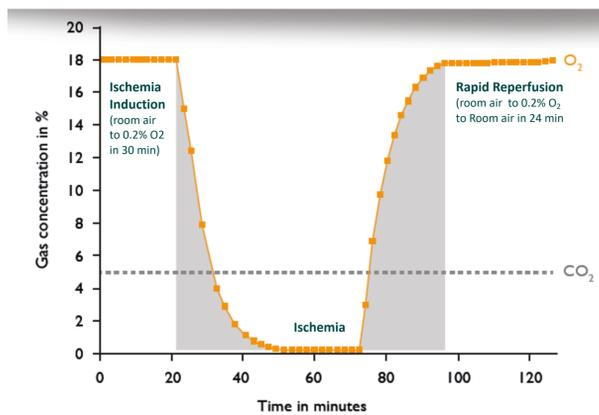
Fig. 1: Sample oxygen ramping and rapid re- of the measurement chamber of a CLARIOstar (BMG Labtech) with integrated ACU. CO<sub>2</sub> can be maintained at 5% during measurement.
